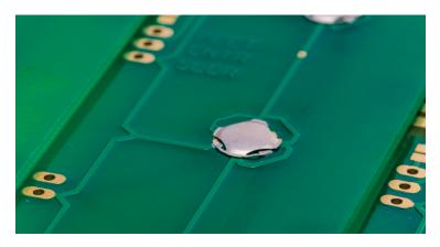
We also recommend considering best flux outgassing practices to ensure contaminate flux deposits are removed during reflow. Please follow recommended procedures from the solder paste or flux manufacturer. Snaptron also recommends allowing at least 50mil separation between the dome and other SMT parts near the dome's solder tabs.
